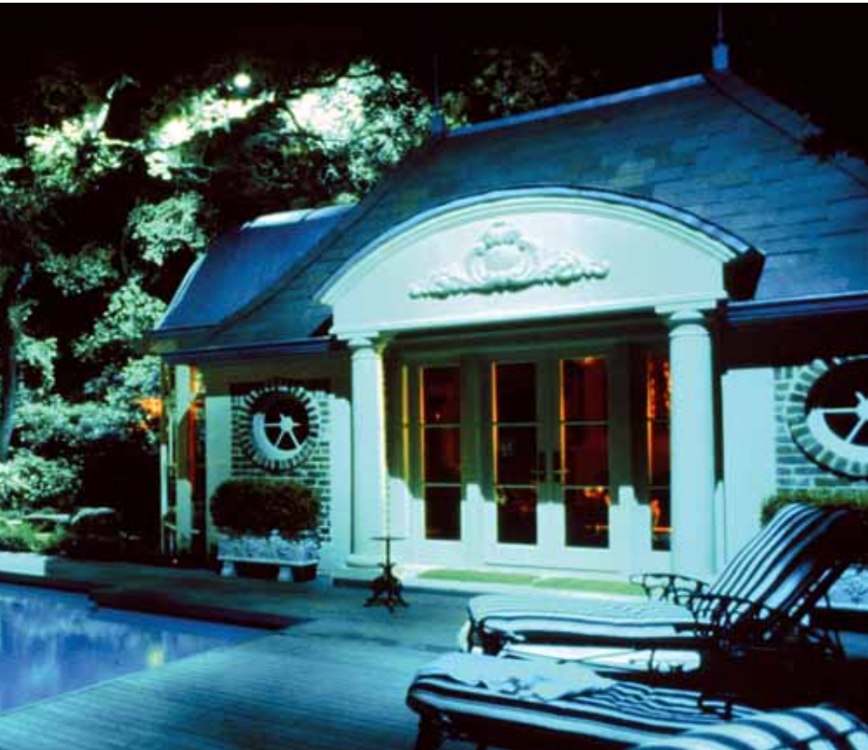
Above Tree mounted bullet downlights with 175-watt MV lamps illuminate pool area.
