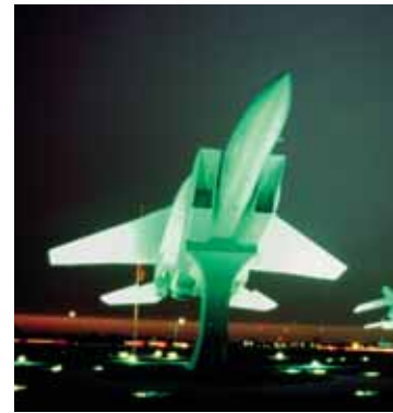
Inground uplights with 175-watt MV lamps light an F-15.
